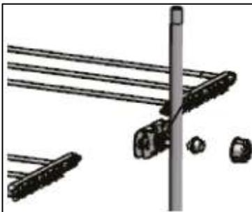
**HANGER (1):** Slide the middle connectors (B) one by one onto the vertical base tube (H) and tighten lightly with the fasteners (I).
