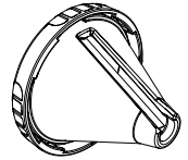
Spiral insert with smooth blade
